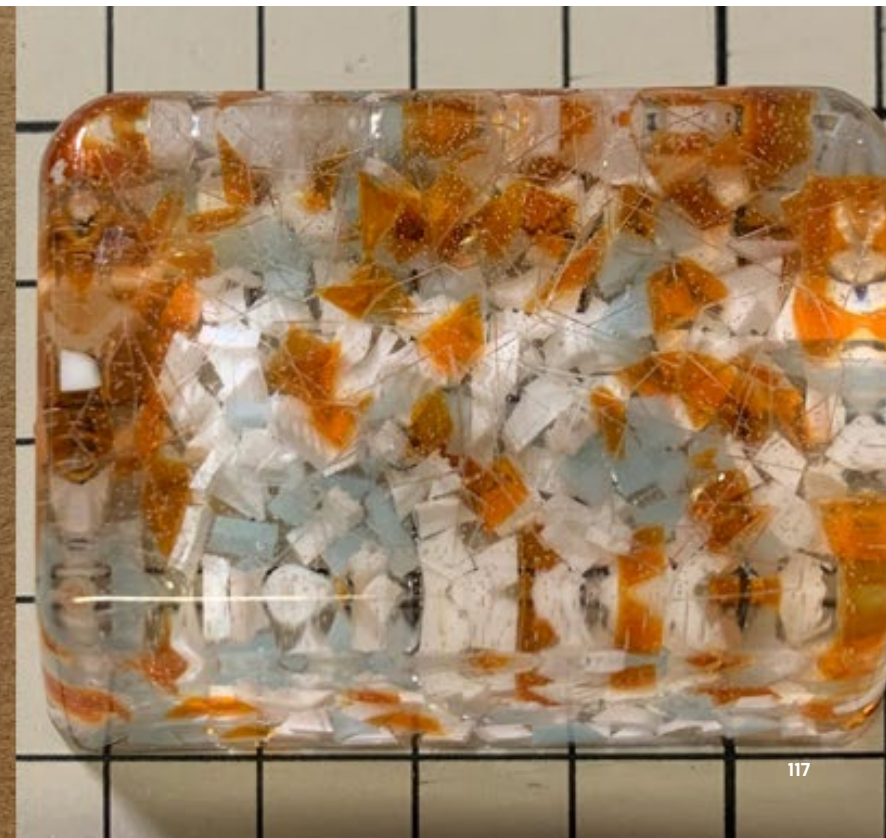
Plastic terrazzo with recycled PET and HDPE by LAU Fong Yui Yvonne
