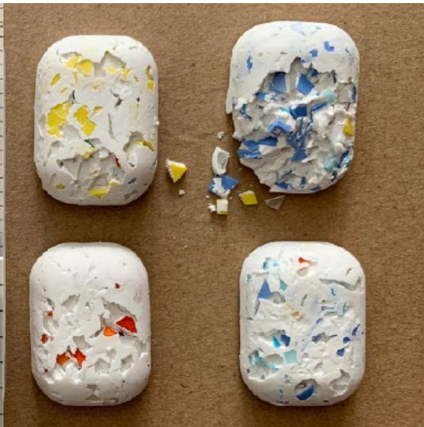
Plastic terrazzo with recycled PET and HDPE by LAU Fong Yui Yvonne
